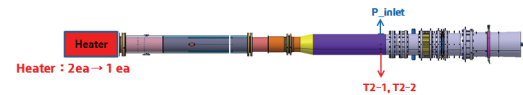
Fig. 15 The configuration of heater and induced pipe of high temperature for M=6.0 .
