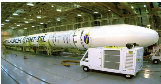
Fig. 3 Integrated launch vehicle in the assembly and command ship[6].
