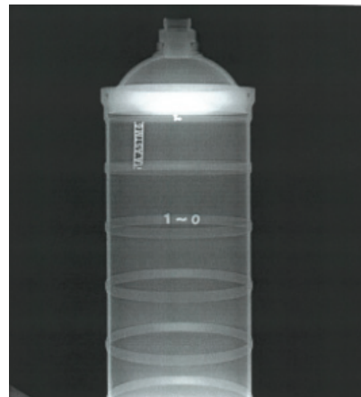
Fig. 8 CR image of propellant 3 - filled tank.
