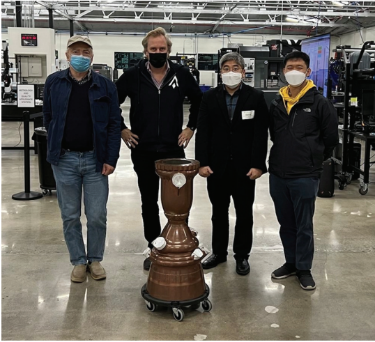
Fig. 10 Launcher's E-2 engine single printed CuCrZr chamber for the Launcher Light rocket.
