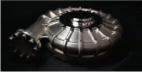
Fig. 5 A 3D printed engine turbopump part of the Archimedes engine[14].
