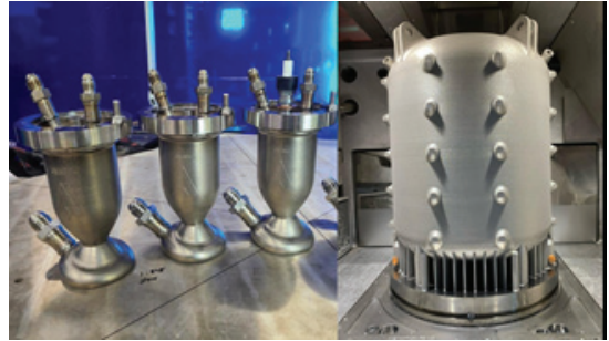
Fig. 11 Orbiter Thrusters (left) and a printed propellant tank (right) for Launcher Orbiter[26].
