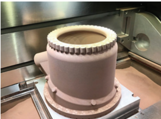
Fig. 14 DemoP1's jacket in the PBF build chamber[33].
