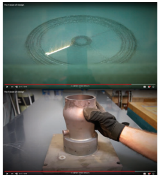
Fig. 1 Manufacturing of main oxygen valve housing of merlin 1D engine[3].
