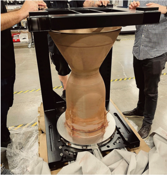
Fig. 7 3D printed copper chamber for the Aeon R engine[19].
