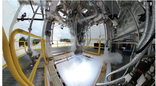
Fig. 6 Combustion test of the 3D printed copper based chamber of the Aeon 1 engine[17].
