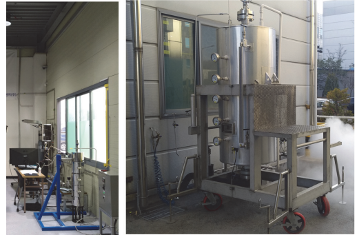
Fig. 12 Testing equipment for propellant tank pressurization.
