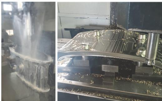
Fig. 2 Image of five-axis machining for the nozzle.
