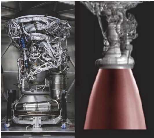
Fig. 9 Merlin 1DV engine without (left) and with extension part (right)[36].
