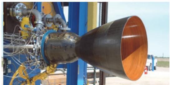
Fig. 6 Kestrel engine doing ablative cooling test[30].
