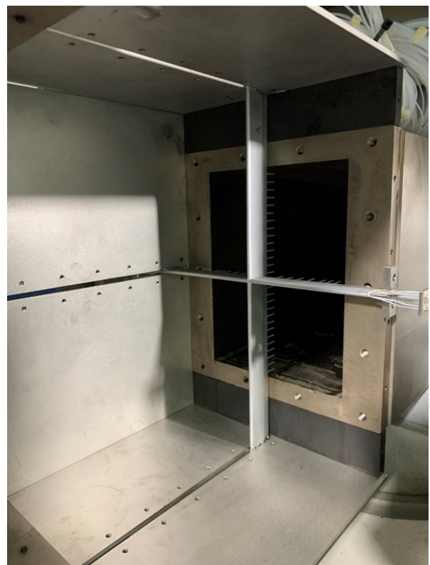
Fig. 7 Picture of Pitot rake installation for new Mach 5 nozzle.
