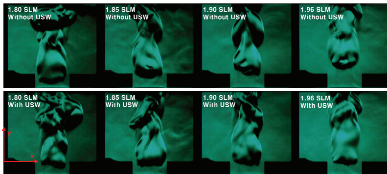
(b) Schlieren image of lifted flames
