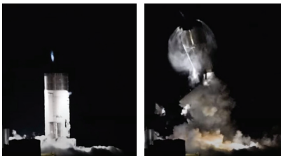
Fig. 14 SN1 destruction during pressure test[19].
