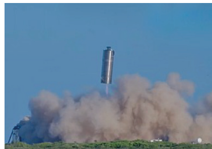
Fig. 16 SN5 during 150 m flight test[19].
