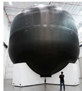
Fig. 3 Initial composite liquid oxygen tank[6].
