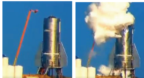
Fig. 12 Mk1 destruction during pressure test[19].
