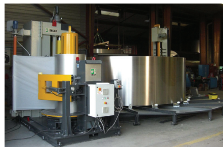
Fig. 13 Bending from rolled sheet to circular barrel[20].
