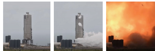
Fig. 15 SN4 explosion after static fire test[19].
