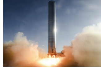
Fig. 18 Super Heavy prototype BN3 static fire test[11].
