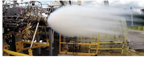
Fig. 9 LOX preburner test at NASA[15].
