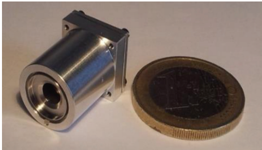
Fig. 22 NanoFEEP thruster compared to a 1 Euro coin[5,50,51].
