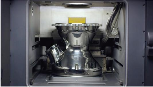
Fig. 4 Part of Aeon 1 engine sits insides a 3D printer [17].
