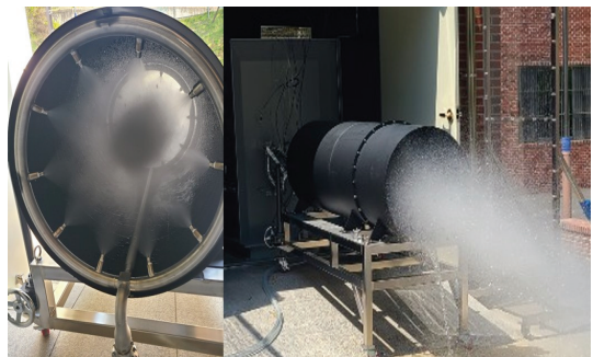
Fig. 7 Operation of the noise suppression system.
