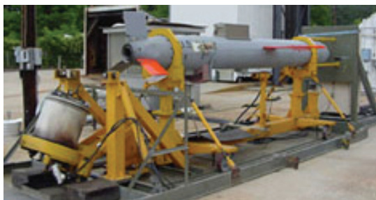
Fig. 11 Ground functional test of propulsion section.
