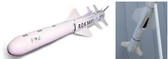
Fig. 5 Dual scoop(Bifurcated) & flush air intake.
