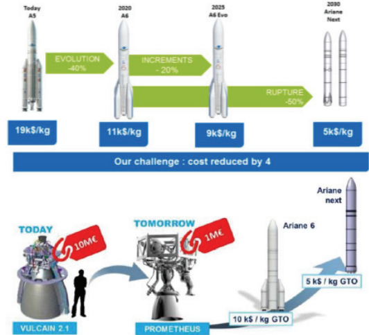
Fig. 20 Evolution plan of ariane launch vehicle and liquid rocket engine[74,75].
