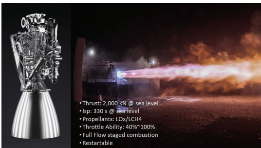
Fig. 5 Raptor Engine Firing Test [40].
