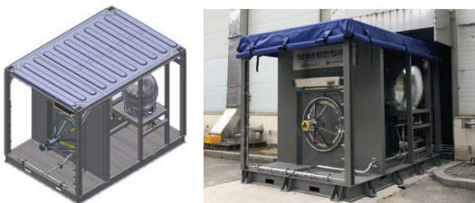
Fig. 43 Hot firing test equipment for methane engine thrust chamber installed in KARI[107].
