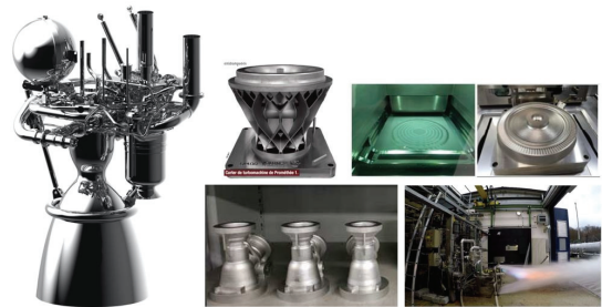
Fig. 21 Prometheus engine, additively manufactured engine components, and test for additively manufactured gas generator at P8 test bench at DLR[74].
