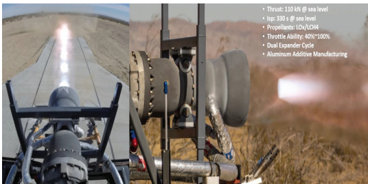
Fig. 13 Firing test of additively manufactured broadsword engine[60].
