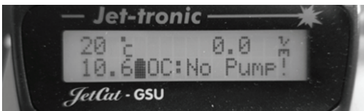
Fig. 16 Fuel pump fault alarm of GSU.
