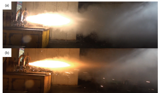
Fig. 4 Test motor plumes with AP/Al propellant (a) GUDN/BTATz propellant (b).
