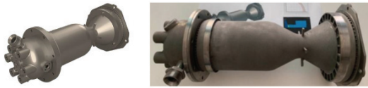
Fig. 8 Thrust chamber made by EBM technology for 5 kN expander cycle engine from CIRA[17].
