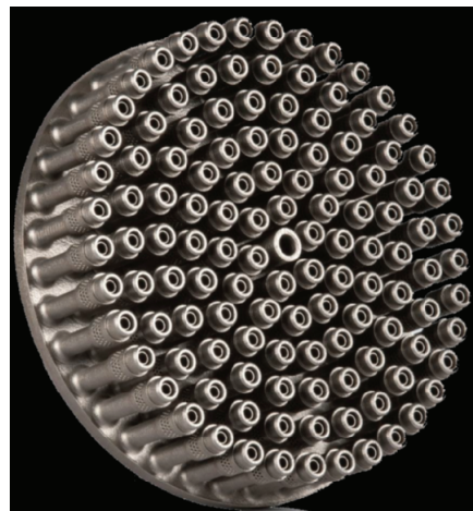
Fig. 5 Injector head consolidation using DMLS for Vinci engine[12].
