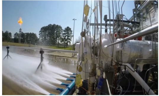
Fig. 11 AM fuel pump test of NASA using LCH4 [21].
