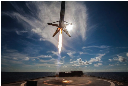
Fig. 7 The first stage of a Falcon 9 v1.2 rocket descends to a landing on SpaceX's drone ship [6].
