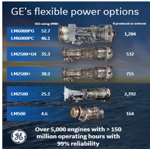
Fig. 3 GE Marine's Aero-Derivative Marine Gas Turbines Line Up.
