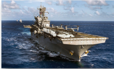
LHD 8: 3.7 MW geared hybrid electric
