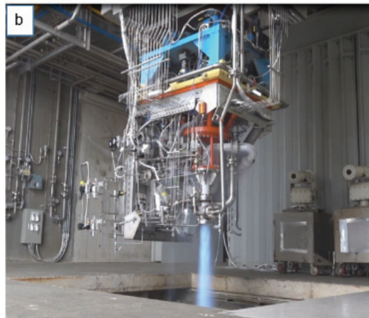
Fig. 5 (a) TDMOB powerpack in test stand and (b) pre-burner combustion.
