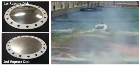
Fig. 4 Rupture disk and Underwater ignition test.
