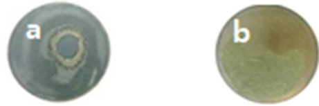
Fig. 9 Coated Specimen after thermal shock (a) EV-300-60M (b) AM-1.
