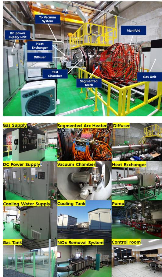
Fig. 1 Measured 0.4 MW class DC arc-heated plasma wind tunnel system.
