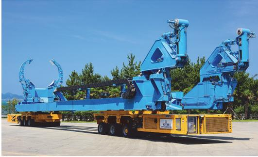
Fig. 6 SPMT and transporter erector for KSLV-I.
