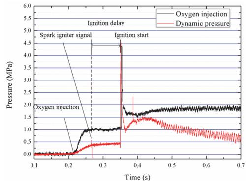
Fig. 6 Calculation method of ignition delay time.
