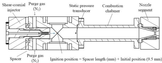
Fig. 2 Schematic of combustor and injector.
