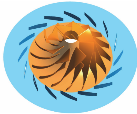
Fig. 11 Geometry of impeller and diffuser vanes.
