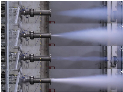
Fig. 7 Combustion test of pre-burner.
