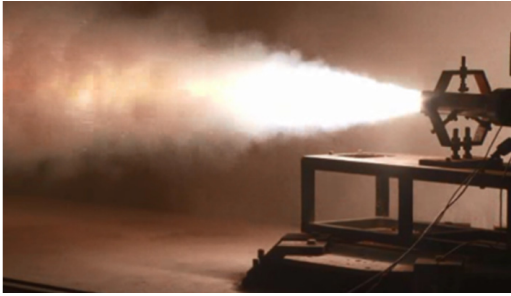
Fig. 3 Ground test for nozzleless booster.
