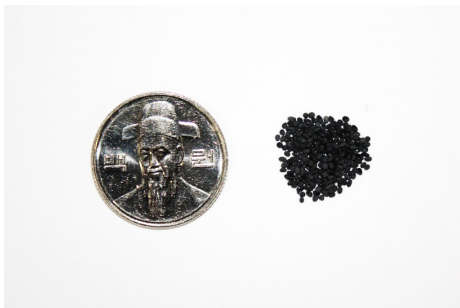
Fig. 4 18-20 Mesh Pt-Cu/LHA catalyst.
