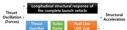
Fig. 1 Closed-loop system of the pogo phenomenon.
