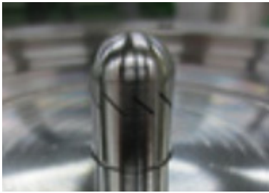
Fig. 18 Canted slit type pintle injector.
