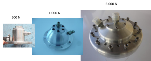
Fig. 11 Pintle injectors designed by the UFMG team.
