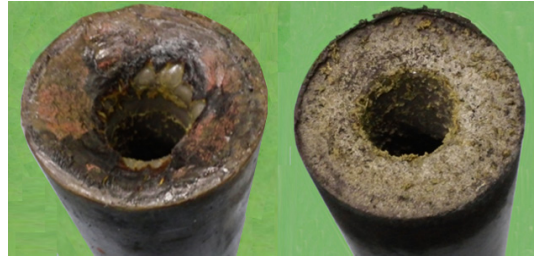
Fig. 13 Fuel grain after ignition test (Left : front side, Right : rear side).
