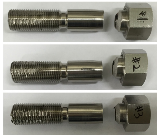
Fig. 6 Results of tensile test.
