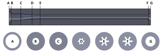
Fig. 2 A schematic picture of NAWC no.6 motor grain.
