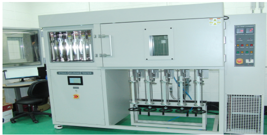
Fig. 4 Strain & Load Endurance Tester in LIGNex1.
