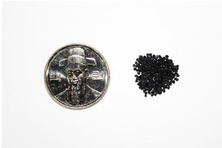
Fig. 4 18-20 Mesh Pt-Cu/LHA catalyst.
