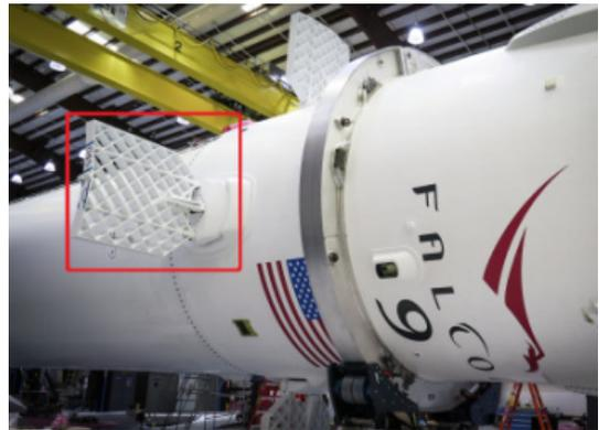
Fig. 14 Grid Fin of Falcon 9[31].
