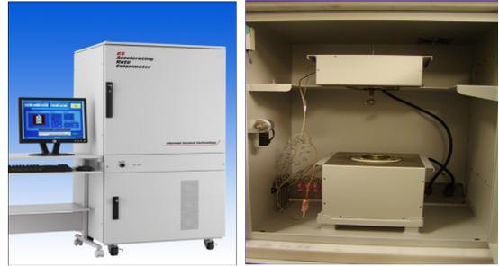
Fig. 10 ARC(Accelerating Rate Calorimeter).
